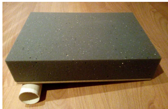
Figure 1. Wood board attached to the PVC tube with foam block on top (before the keel was cut).
